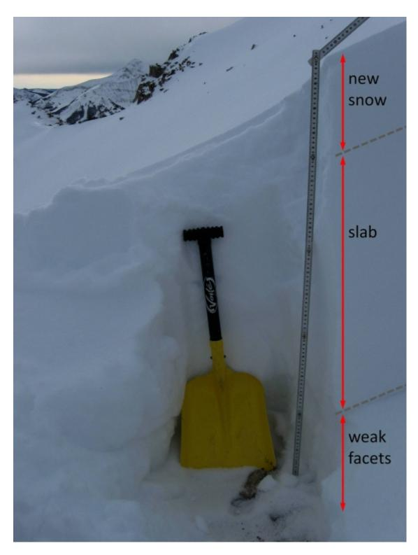
Thin snow equals weak snow. This photo was taken near Big Sky at the head of Middle Basin on a broad planar slope which faces south and southeast. Without a significant load of new snow, triggerring an avalanche in these areas isn't likely but should be considered. Stability test results on the facets were CT20 Q1 and ECTP20. Find a deeper snowpack, and you will find much stronger snow. Photo: GNFAC
