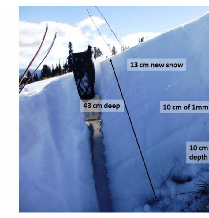
The snowpack around Lionhead (8,000') was only 43 cm deep. It was faceted with the larger crystals at the ground. I got no collapsing or cracking as I skied around. Once more snow falls I expect the snowpack to quickly become unstable. Photo: GNFAC
