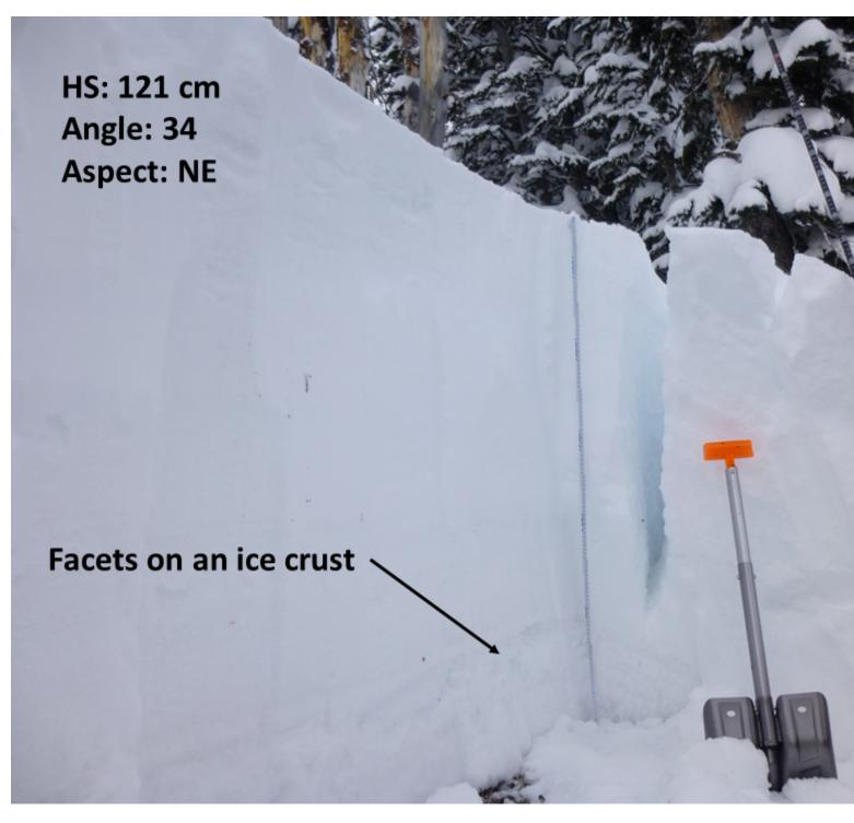
The avalanche broke on a layer of well-developed facets that are sitting on an ice crust. The crack in the snowpit wall is a remnant slab that cracked, but did not slide down the hill in the avalanche. Photo: GNFAC
